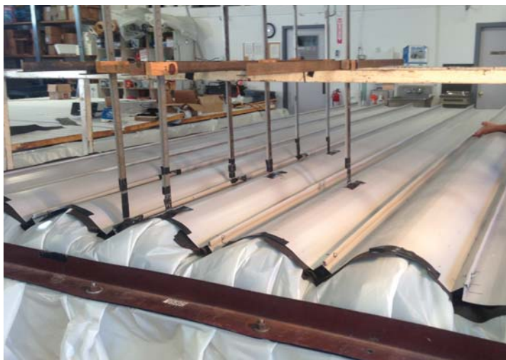
ATSM E 1592 test with pressure being applied.
