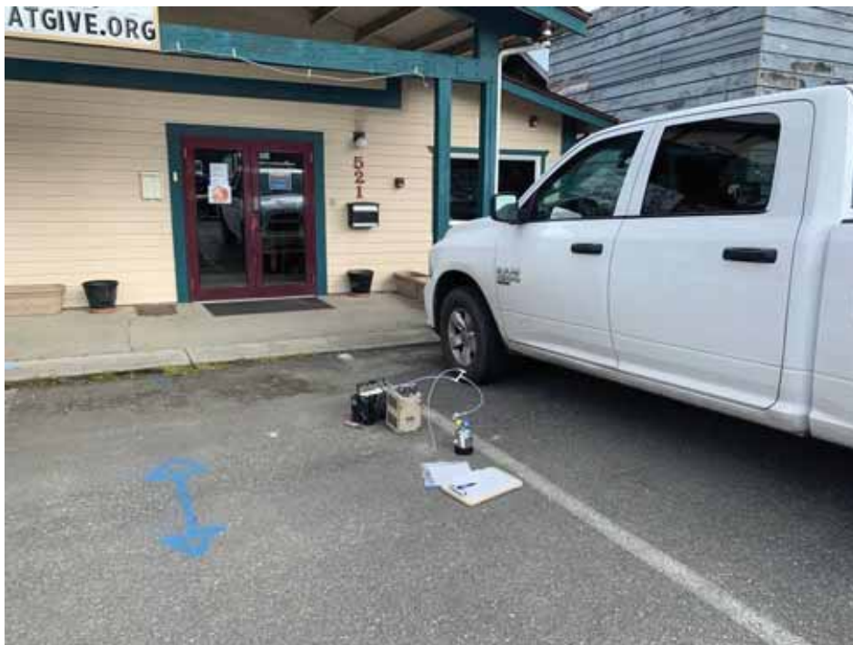
Photo 2: Subject Site – View showing vapor probe location VP-2 in front of 521 Bay Street. This photo shows the sampling set-up.
