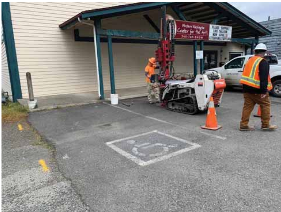
Photo 6: Subject Site – View showing soil boring location B-4 in front of 521 Bay Street. This was located near the location of the former heating oil UST.
